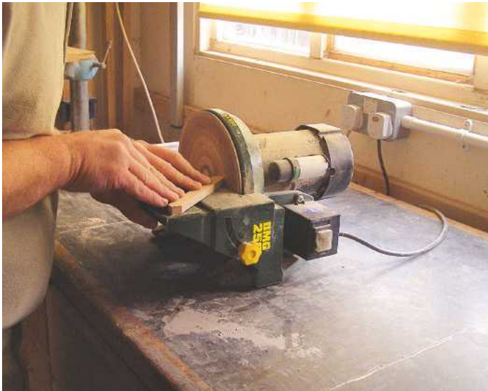
▲ Pic.10 Carefully sand the infill rails to length and to the correct angles. Make sure the table is set square to the sanding disc
